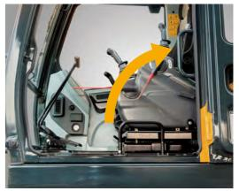
New joystick grips for precise control have been equipped with double switches. - Left: One touch deceleration
