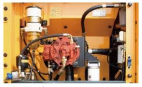
Hydraulic oil filter chip replacement cycle is extended (1,000 hours).
