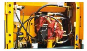
To achieve optimum precision, Hyundai redesigned the hydraulic system to provide the operator with super fine touch and top level controllability. Spool valves in the control valve are engineered to provide more precise flow to each function with less effort.
